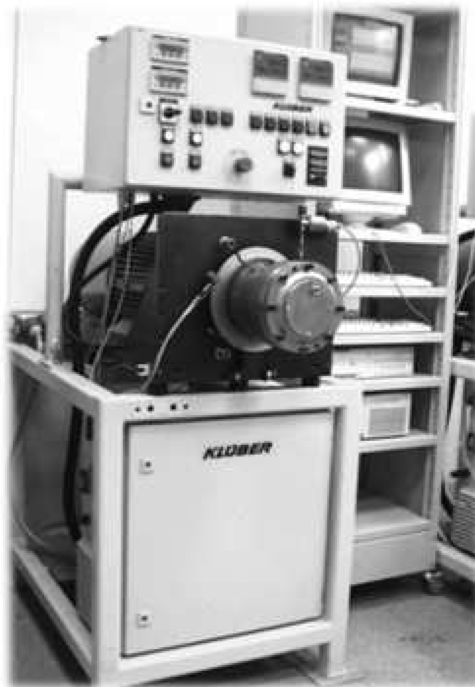
FAG FE8 wear test
