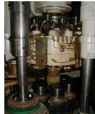
A grease lubrication system on a Can Seaming machine
