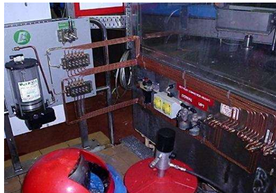
A total loss grease lubrication system under installation on a filling machine in the food industry
