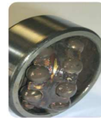
Used Paper Industry Dryer Bearing
