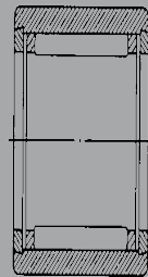
NK - Needle Roller Bearings with flanges, without inner ring
