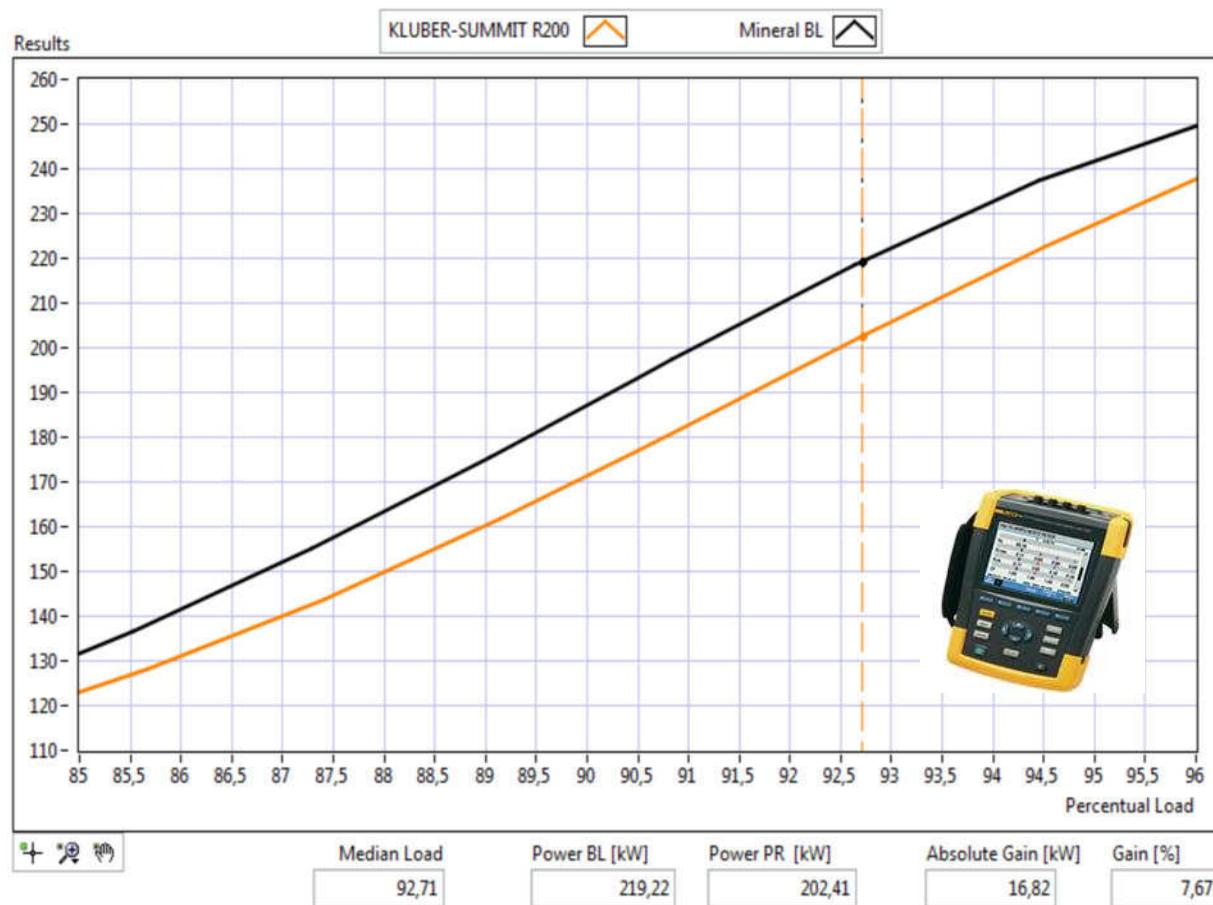
Knowing the Power Factor from the motor, we can get the load of the compressor load (in %) at any moment and matching it with the real KWh demanded.
