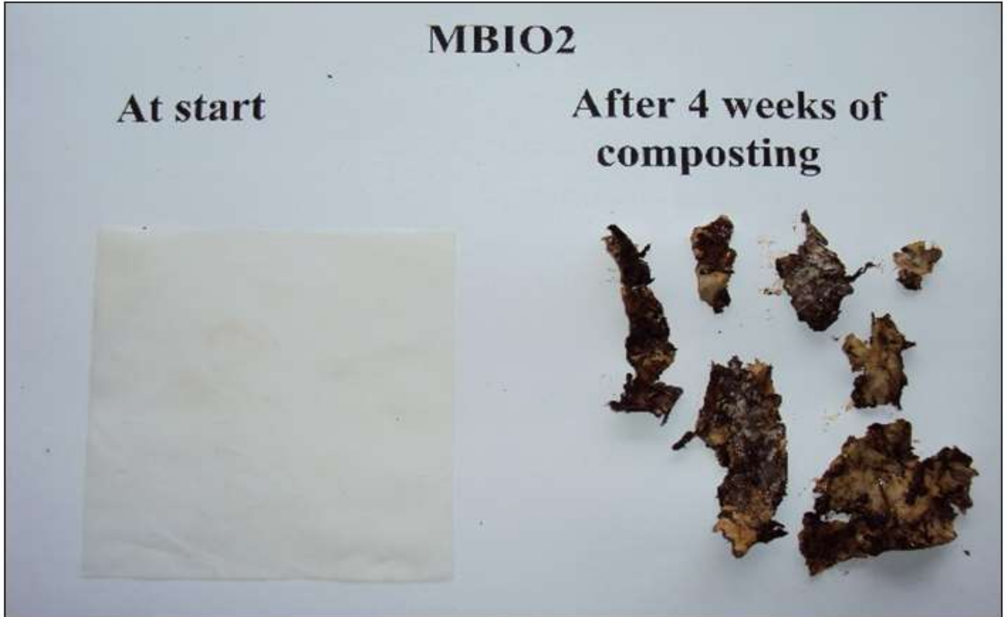
Figure 13. Visual comparison between test item MBIO-2 at start and after 4 weeks of composting.
