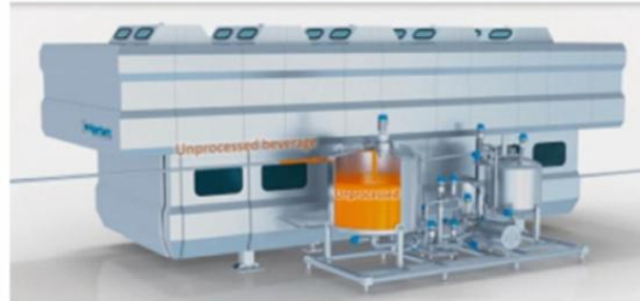
3- Pressurization up to 87,000 psi (600 MPa) during few minutes
