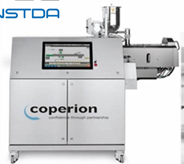
Co-rotating Twin Screw Extruder (ZSK 18MEGAlab, Coperion, Germany)
