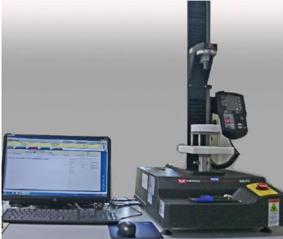
Universal Testing Machine (Instron 5943) Load capacity: 1, 100, 1,000 N load cells
